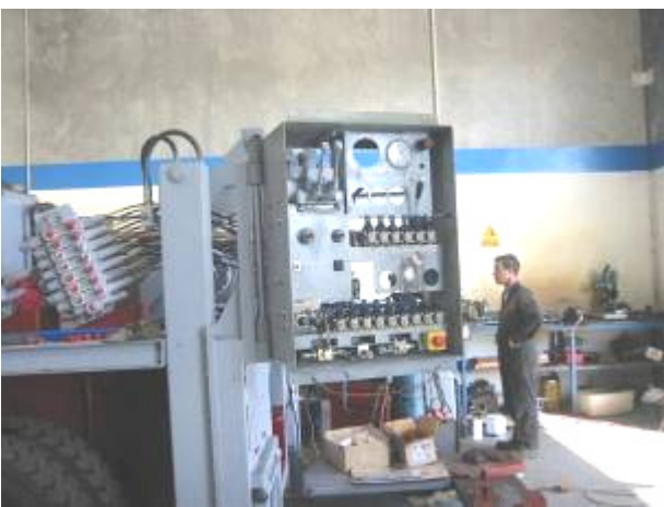
Swinging operator station moves controls away from compressed air dischargers.
