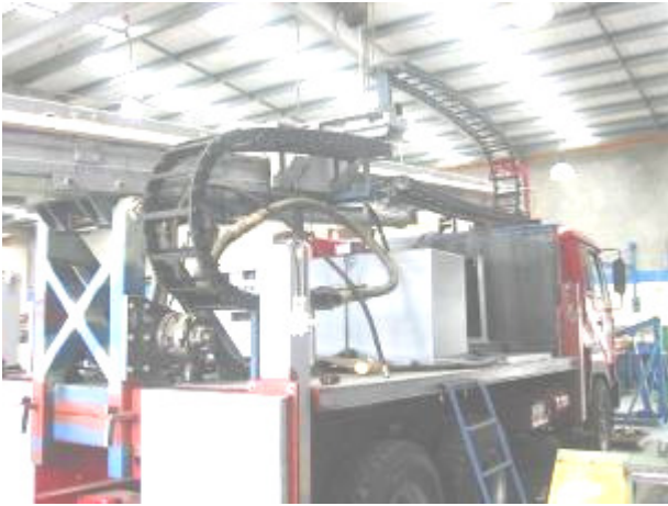
Running hydraulic lines so they remain 'captured' whatever the drill head position.
